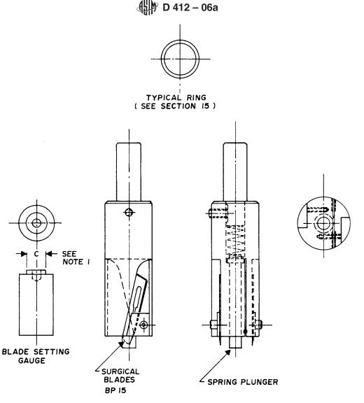
Note—Dimension C to be 2 mm (0.08 in.) less than the inside diameter of the ring. FIG. 3 Typical Ring Cutter Assembly
