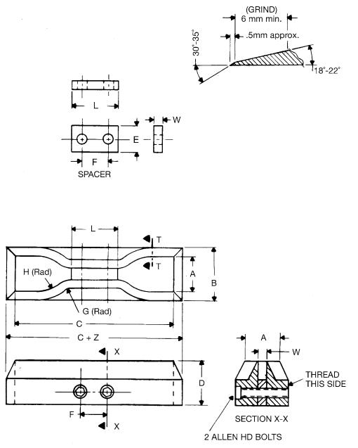
FIG. 2 Standard Dies for Cutting Dumbbell Specimens
